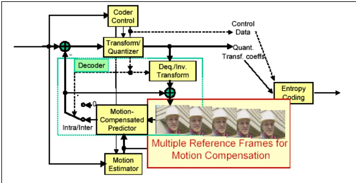
Figure 4. Multiple reference frames
