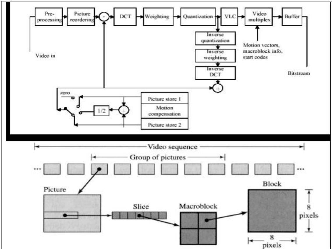
Figure 2. MPEG-2 encoding
